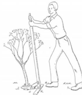
the lifter arm behind the jaw and giving the grip handle a tug. If the jaw shows any tendency to slip upward instead of gripping the stem, keep pressure with your foot on the lifter arm until the jaw is solidly clamped on.
