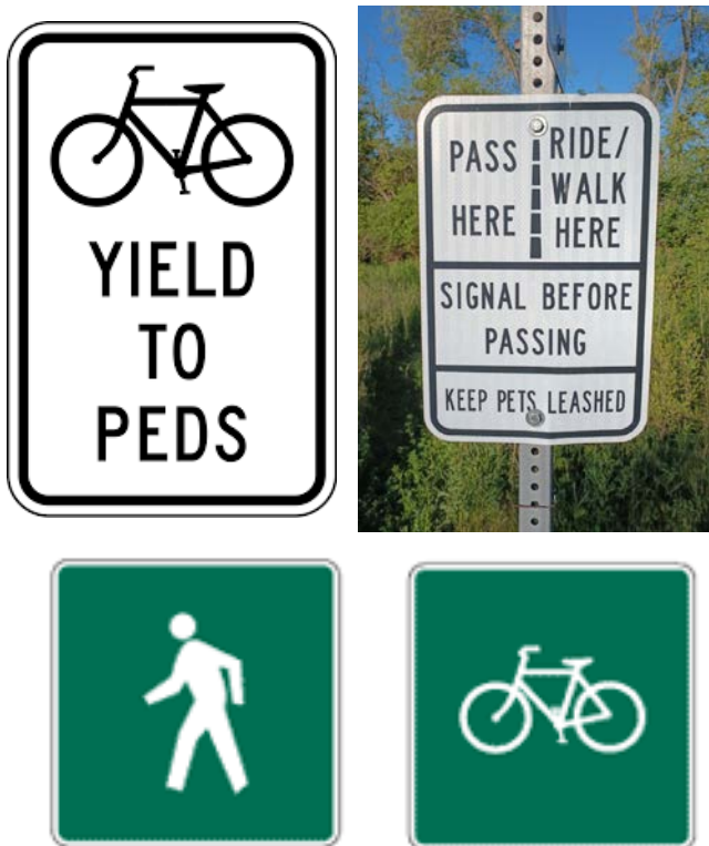
Figure 3.6: Examples of path signs to encourage proper yielding, sharing, and signaling include “Bicyclists Yield to Pedestrians” MUTCD R9-6 signs (left), “Pedestrians and Bicyclists Permitted” MUTCD D11-2 and D11-1a (bottom), and tailored messaging as shown in this example from Cedar Rapids, IA (right).
